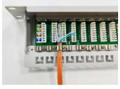
7. Connect the wires starting from clamp 8 using the LSA connection tool.
