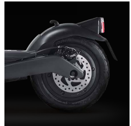
Front and rear disc brake with KERS
