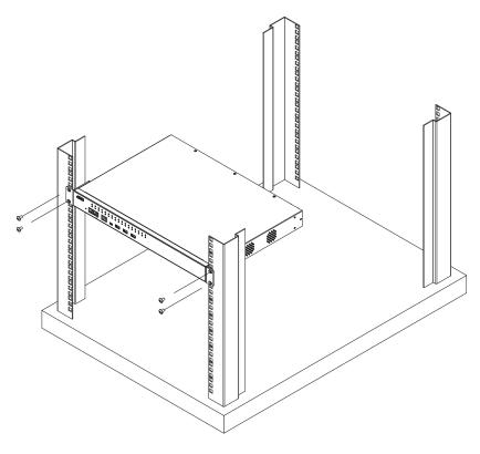
**Note:** Cage nuts are provided for racks that are not pre-threaded.
