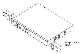
3. Position the device in the front of the rack and align the holes in the mounting brackets with the holes in the rack. Screw the mounting brackets to the rack.
