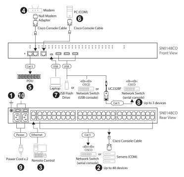
**Note:** A SN0148CO serial console server is used as an example to illustrate the installation. As for other serial console servers, the installation is identeical with fewer serial ports.
