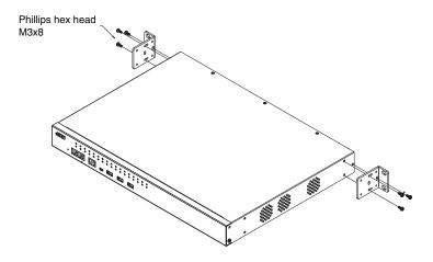
3. Position the device in the rack and align the holes in the mounting brackets with the holes in the rack.
